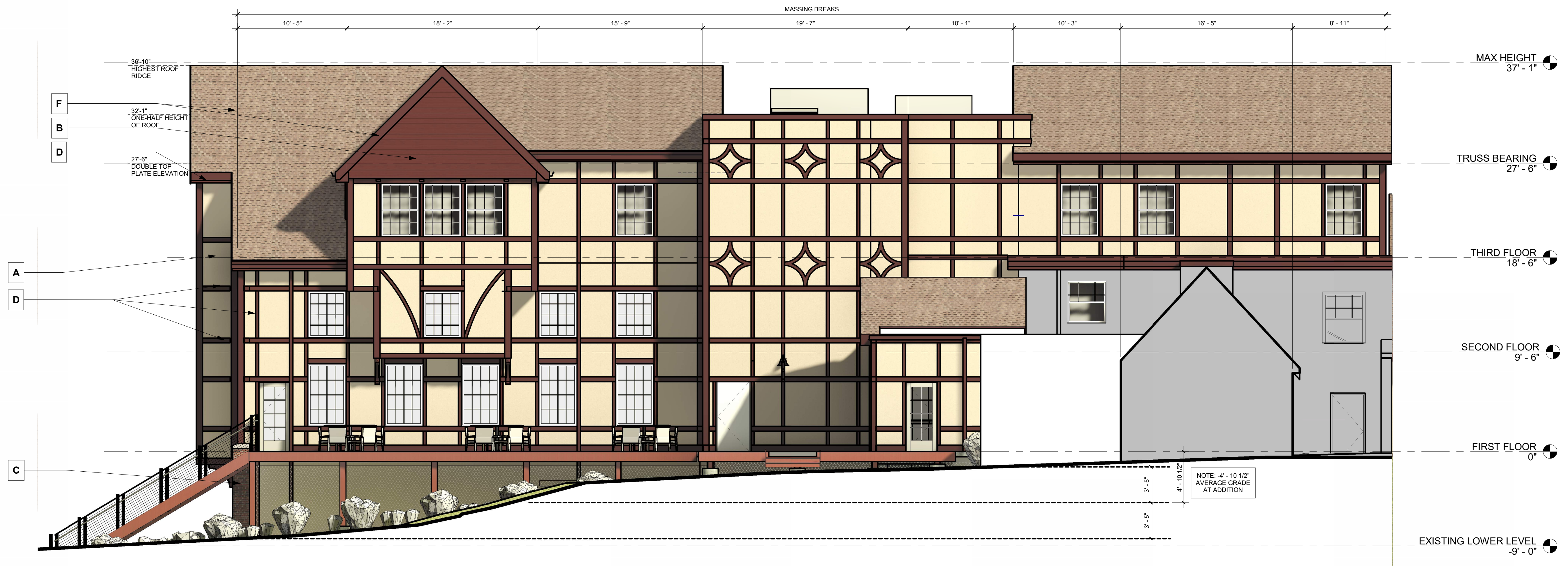
1 MEN'S WING EXTERIOR WEST ELEVATION - RENDERED A303 3/16" = 1'-0"
