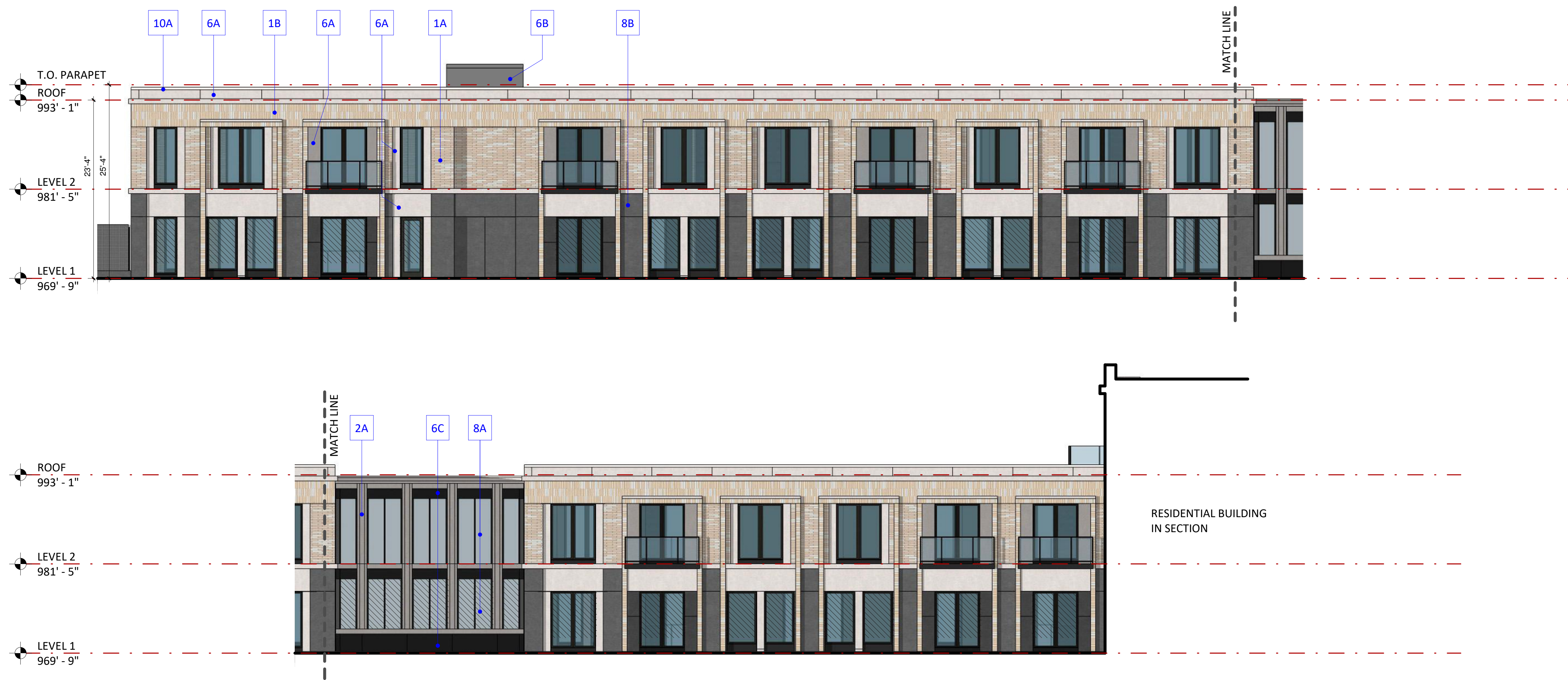
1 COURTYARD ELEVATION - NORTH MP0.11 1/8" = 1'-0"
